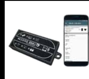
Access BMU Battery-Monitoring-Unit
