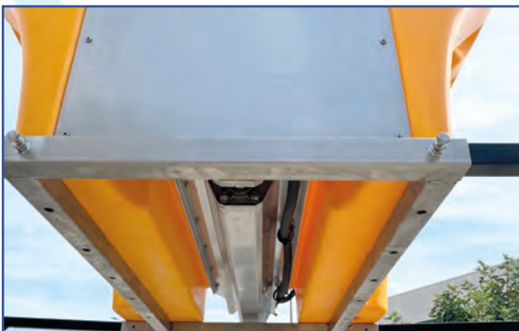
Salt spreader structure in double-walled PPL, stainless steel auger flow channel and auger
